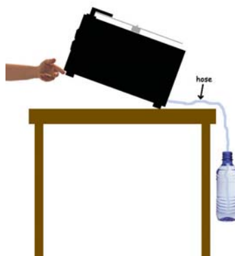
Photo 6: draining the cleaning liquid
