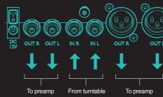
Once Huei is connected, do not switch your preamp/amplifier 'on' until the volume is at its lowest setting. Next, turn Huei 'on' and select the appropriate settings for your cartridge as explained below. With the settings correct, select the lowest gain setting on Huei (white), before turning connected equipment 'on'. Next, select the appropriate input on your preamplifier, begin playing the source and gradually increase the gain/volume to a comfortable level.
